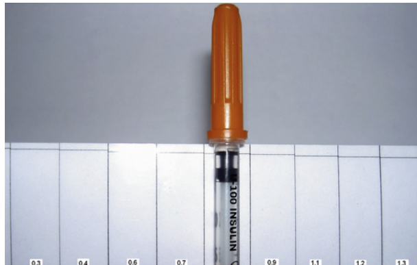
Fig. 1. An insulin syringe filled to 0.8 IU using an insulin syringe ruler. The ruler has been calibrated for BD Micro-Fine+ Demi 0.3-mL U-100 syringes (Becton Dickinson, Franklin Lakes, NJ), containing half unit markings, widely available in Germany, Switzerland, and Austria. The ruler is available for download at the following address: http://www.diabetes-katzen.net/insulinruler.pdf . Note that in Europe, a comma is commonly used instead of a decimal point. The syringes themselves are printed with 0,3 mL, and the packaging for the syringes is also labeled 0,3 mL.
